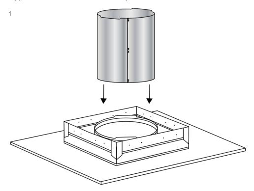
Connect the tube to the ring with the interlocking connecting clips as shown below.
