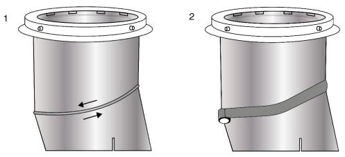
Now remove the transparent protective film from the inside of the top tube assembly.
