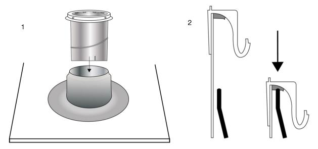
**Note:** The insulator is designed to fit tightly around the outside of the tube, so you may have to stretch the insulator with your finger tips to allow the tube to fit through.
