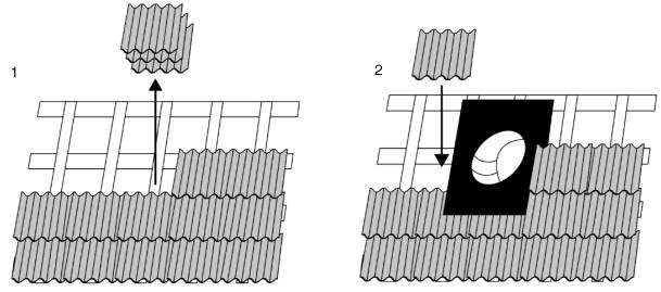
**Tip:** The bottom skirt of the Ubiflex flashing is longer than the top.
