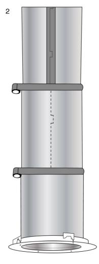
Slide the tube up through the opening in the ceiling from below.
