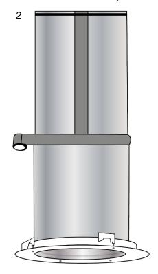
Slide the tube up through the opening in the ceiling from below.
