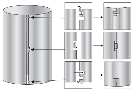
Tape the entire length of the tube seam with aluminum tape on the outside of the tube. Remove the protective film from the extension tube
