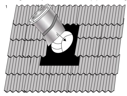
Fix the dome ring onto the roof flashing using the dome screws provided, screwed through the four grey spacers from the outside in. The screws will pierce through the flashing and the inside of the reflective tubing. Be careful not to overtighten the screws as this may cause damage to the dome ring.
