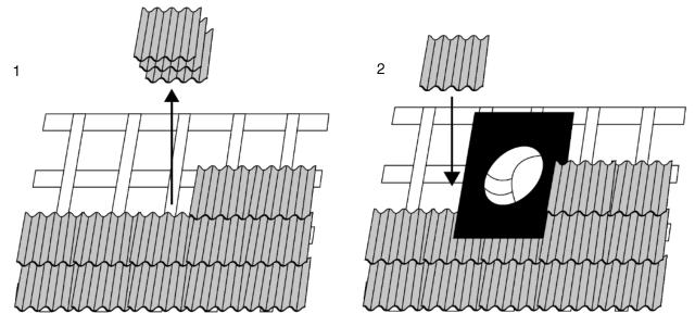
**Tip:** The bottom skirt of the Ubiflex flashing is longer than the top. Fix the Ubiflex roof flashing in place by screwing the top of the flashing to the tile battens.
