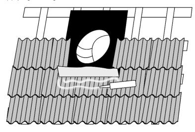
Fit the roof tiles back around the sides and top of the roof flashing.
